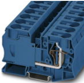
Feed-through terminal block, Connection method: Spring-cage connection, Cross section: 2.5 mm 2 - 35 mm 2 , AWG: 14 - 2, Width: 16 mm, Color: blue, Mounting type: NS 35/7,5, NS 35/15
