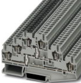
Multi-level terminal block, Connection method: Spring-cage connection, Cross section: 0.08 mm 2 - 4 mm 2 , AWG: 28 - 12, Width: 5.2 mm, Color: gray, Mounting type: NS 35/7,5, NS 35/15
