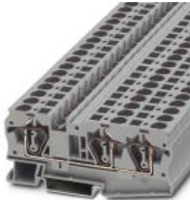
Feed-through terminal block, Connection method: Spring-cage connection, Cross section: 0.2 mm 2 - 10 mm 2 , AWG: 24 - 8, Width: 8.2 mm, Color: blue, Mounting type: NS 35/7,5, NS 35/15
