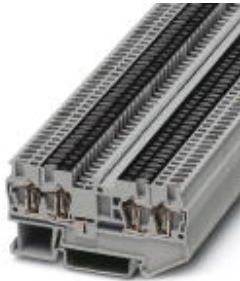
Feed-through terminal block, Connection method: Spring-cage connection, Cross section: 0.08 mm 2 - 1.5 mm 2 , AWG: 28 - 16, Width: 4.2 mm, Color: gray, Mounting type: NS 35/7,5, NS 35/15
