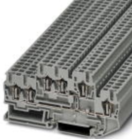
Feed-through terminal block, Cross section: 0.08 mm 2 - 4 mm 2 , AWG: 28 - 12, Connection type: Spring-cage connection, Width: 5.2 mm, Color: gray, Mounting type: NS 35/7,5, NS 35/15
