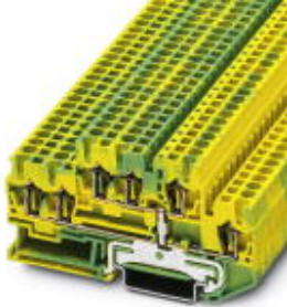
Feed-through terminal block, Cross section: 0.08 mm 2 - 4 mm 2 , AWG: 28 - 12, Connection type: Spring-cage connection, Width: 5.2 mm, Color: green-yellow, Mounting type: NS 35/7,5, NS 35/15
