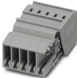
Coupling, Connection method: Plug connection, Number of positions: 8, Cross section: 0.08 mm 2 - 4 mm 2 , AWG: 28 - 12, Width: 41.6 mm, Height: 18.8 mm, Color: gray
