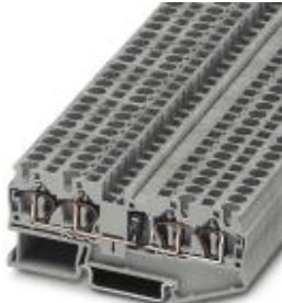
Component terminal block, Connection method: Spring-cage connection, Cross section: 0.08 mm 2 - 6 mm 2 , AWG: 28 - 10, Width: 6.2 mm, Color: gray, Mounting type: NS 35/7,5, NS 35/15
