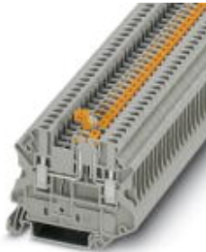
Knife disconnect terminal block, Connection method: Screw connection, Cross section: 0.14 mm 2 - 4 mm 2 , AWG: 26 - 12, Width: 5.2 mm, Color: gray, Mounting type: NS 35/7,5, NS 35/15
