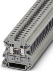
Feed-through terminal block, Connection method: Screw connection, Cross section: 0.14 mm 2 - 6 mm 2 , AWG: 26 - 10, Width: 6.2 mm, Color: brown, Mounting type: NS 35/7,5, NS 35/15
