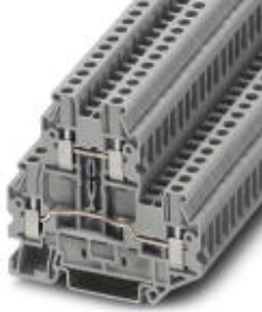
Double-level terminal block, Cross section: 0.14 mm 2 - 4 mm 2 , AWG: 26 - 12, Connection type: Screw connection, Width: 5.2 mm, Color: gray, Mounting type: NS 35/7,5, NS 35/15
