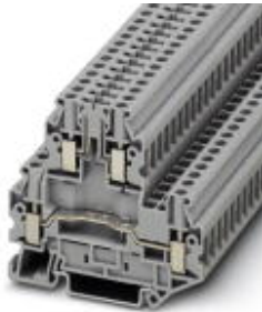
Disconnect terminal block, Cross section: 0.14 mm 2 - 6 mm 2 , AWG: 26 - 10, Connection type: Screw connection, Width: 6.2 mm, Color: gray, Mounting type: NS 35/7,5, NS 35/15
