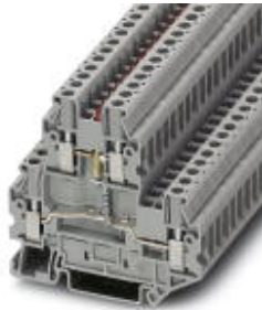
Component terminal block, Cross section: 0.14 mm 2 - 4 mm 2 , AWG: 26 - 12, Connection type: Screw connection, Width: 5.2 mm, Color: gray, Mounting type: NS 35/7,5, NS 35/15
