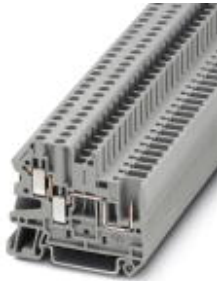
Feed-through terminal block, Connection method: Screw/plug-in connection, Cross section: 0.14 mm 2 - 6 mm 2 , AWG: 26 - 10, Width: 6.2 mm, Color: gray, Mounting type: NS 35/7,5, NS 35/15
