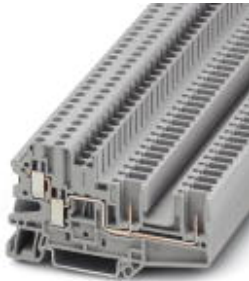
Feed-through terminal block, Connection method: Screw/plug-in connection, Cross section: 0.14 mm 2 - 6 mm 2 , AWG: 26 - 10, Width: 6.2 mm, Color: gray, Mounting type: NS 35/7,5, NS 35/15
