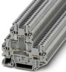
Feed-through terminal block, Cross section: 0.14 mm 2 - 4 mm 2 , AWG: 26 - 12, Connection type: Screw connection, Width: 5.2 mm, Color: gray, Mounting type: NS 35/7,5, NS 35/15
