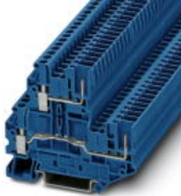
Double-level terminal block, Cross section: 0.14 mm 2 - 4 mm 2 , AWG: 26 - 12, Connection type: Screw/plug-in connection, Width: 5.2 mm, Color: blue, Mounting type: NS 35/7,5, NS 35/15
