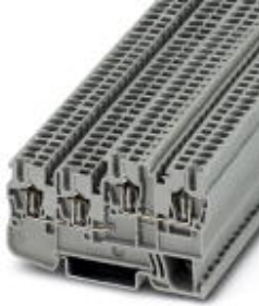
Sensor/actuator terminal block, Connection method: Spring-cage connection, Cross section: 0.08 mm 2 - 4 mm 2 , AWG: 28 - 12, Width: 5.2 mm, Color: gray, Mounting type: NS 35/7,5, NS 35/15
