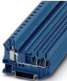
Feed-through terminal block, Connection method: Screw connection, Cross section: 0.5 mm 2 - 16 mm 2 , AWG: 20 - 6, Width: 10.3 mm, Color: blue, Mounting type: NS 35/7,5, NS 35/15
