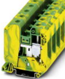
Feed-through terminal block, Connection method: Screw connection, Cross section: 1.5 mm 2 - 50 mm 2 , AWG: 16 - 2, Width: 16 mm, Color: green-yellow, Mounting type: NS 35/7,5, NS 35/15
