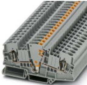
Test disconnect terminal block, Connection method: Spring-cage connection, Cross section: 0.2 mm 2 - 10 mm 2 , AWG: 24 - 8, Width: 8.2 mm, Color: gray, Mounting type: NS 35/7,5, NS 35/15
