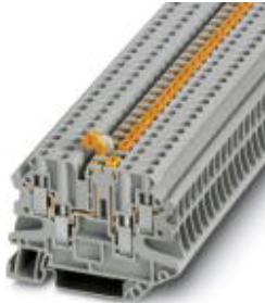
Knife disconnect terminal block, Connection method: Screw connection, Cross section: 0.14 mm 2 - 6 mm 2 , AWG: 26 - 10, Width: 6.2 mm, Color: gray, Mounting type: NS 35/7,5, NS 35/15
