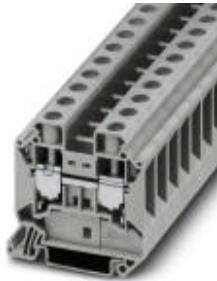
Feed-through terminal block, Connection method: Screw connection, Cross section: 1.5 mm 2 - 25 mm 2 , AWG: 16 - 4, Width: 12.2 mm, Color: orange, Mounting type: NS 35/7,5, NS 35/15
