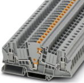
Test disconnect terminal block, Connection method: Screw connection, Cross section: 0.2 mm 2 - 10 mm 2 , AWG: 24 - 8, Width: 8.2 mm, Color: gray, Mounting type: NS 35/7,5, NS 35/15
