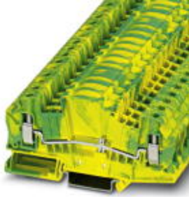
Ground modular terminal block, Connection method: Screw connection, Cross section: 0.2 mm 2 - 10 mm 2 , AWG: 24 - 8, Width: 8.2 mm, Color: green-yellow, Mounting type: NS 35/7,5, NS 35/15
