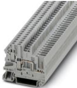
Feed-through terminal block, Connection method: Screw/plug-in connection, Cross section: 0.14 mm 2 - 4 mm 2 , AWG: 26 - 12, Width: 5.2 mm, Color: gray, Mounting type: NS 35/7,5, NS 35/15
