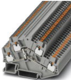
Double-level terminal block, Cross section: 0.14 mm 2 - 4 mm 2 , AWG: 26 - 12, Connection type: Push-in connection, Width: 5.2 mm, Color: gray, Mounting type: NS 35/7,5, NS 35/15
