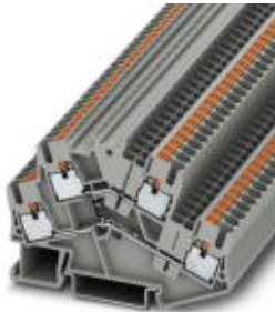
Component terminal block, Connection method: Push-in connection, Cross section: 0.14 mm 2 - 4 mm 2 , AWG: 26 - 12, Width: 5.2 mm, Color: gray, Mounting type: NS 35/7,5, NS 35/15
