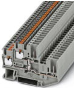
Double-level terminal block, Cross section: 0.14 mm 2 - 4 mm 2 , AWG: 26 - 12, Connection type: Push-in / plug connection, Width: 5.2 mm, Color: gray, Mounting type: NS 35/7,5, NS 35/15
