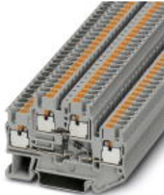
Feed-through terminal block, Cross section: 0.14 mm 2 - 4 mm 2 , AWG: 26 - 12, Connection type: Push-in connection, Width: 5.2 mm, Color: gray, Mounting type: NS 35/7,5, NS 35/15
