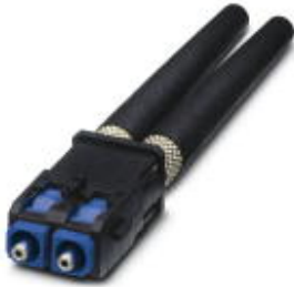
SCRJ fiber optic connector, IP20, duplex, with fast connection technology, for polymer fiber 980/1000 µm, for individual wire diameter 2.2 mm
