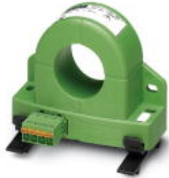
Universal current transducer, for measuring DC, AC, and distorted currents, 0 ... 100 A input current, 0 ... 10 V output
