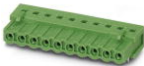
Header, Nominal current: 12 A, Rated voltage (III/2): 320 V, Number of positions: 12, Pitch: 5.08 mm, Color: green, Contact surface: Tin, Assembly: Soldering
