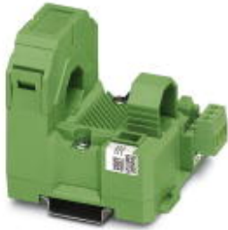
MCR current measuring transducer, for measuring sinusoidal and non-sinusoidal alternating currents, input current 0...400 A, output voltage 0...(5) 10 V
