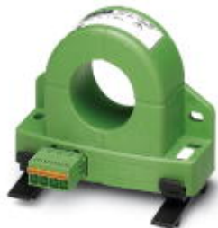
Universal current transducer, for measuring DC, AC, and distorted currents, 0 ... 200 A input current, 0 ... 10 V output
