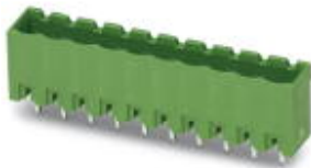
Header, Nominal current: 12 A, Rated voltage (III/2): 320 V, Number of positions: 14, Pitch: 5 mm, Color: green, Contact surface: Tin, Assembly: Soldering
