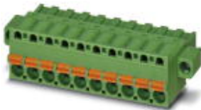
Plug component, Nominal current: 12 A, Rated voltage (III/2): 320 V, Number of positions: 10, Pitch: 5.08 mm, Connection method: Spring-cage conn., Color: green, Contact surface: Tin
