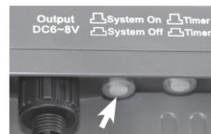
9. The operating voltage of the pump may be adjusted to 6 V and 8 V. This is done by means of a controller. Thus, the power of the pump is adjustable.
