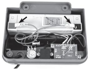
We recommend to exchange the accumulator approx. every 2 years. A new identical in construction accumulator is available from the manufacturer or dealer.
