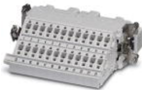
HEAVYCON terminal adapter, pin insert, B24 series, 24-pos., for the right side of the control cabinet, push-in connection
