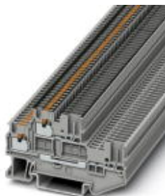
Double-level terminal block, Cross section: 0.14 mm 2 - 1.5 mm 2 , AWG: 26 - 14, Connection type: Push-in / plug connection, Width: 3.5 mm, Color: gray, Mounting type: NS 35/7,5, NS 35/15
