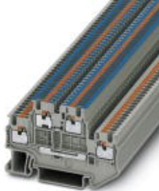
Double-level terminal block, Cross section: 0.14 mm 2 - 1.5 mm 2 , AWG: 26 - 14, Connection type: Push-in connection, Width: 3.5 mm, Color: gray, Mounting type: NS 35/7,5, NS 35/15
