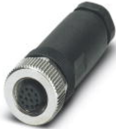
Connector, Universal, 12-position, Socket straight M12, A-coded, Solder connection, Knurl material: Zinc die-cast, nickel-plated, Cable gland Pg9, External cable diameter 6 mm ... 8 mm
