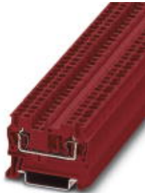
Feed-through terminal block, Connection method: Spring-cage connection, Cross section: 0.08 mm 2 - 4 mm 2 , AWG: 28 - 12, Width: 5.2 mm, Color: red, Mounting type: NS 35/7,5, NS 35/15
