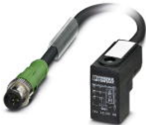
Sensor/Actuator cable, 3-position, PUR halogen-free, Black-gray RAL 7021, Plug straight M12 SPEEDCON, A-coded, on Valve connector C (8 mm), with 1 LED, connected with Z diode, Cable length: 3 m
