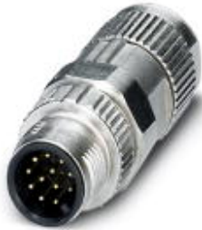
Sensor/actuator connector, male connector, straight, 12-pos., M12 SPEEDCON, metal knurl, Piercecon®, maximum cable diameter of 8.2 mm
