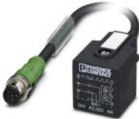
Sensor/Actuator cable, 3-position, PUR halogen-free, Black-gray RAL 7021, Plug straight M12, A-coded, on Valve connector A, with 1 LED, connected with Z diode, Cable length: 3 m
