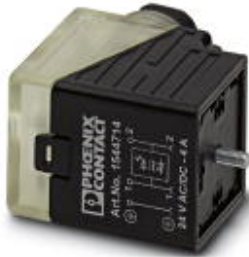
Valve connector, 3-pos., type A, 1 LED, with protective circuit, screw connection, cable screw connection M16
