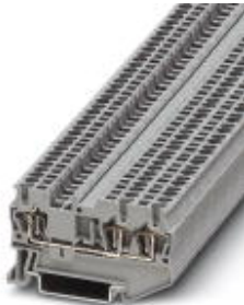
Feed-through terminal block, Connection method: Spring-cage connection, Cross section: 0.08 mm 2 - 1.5 mm 2 , AWG: 28 - 16, Width: 4.2 mm, Color: black, Mounting type: NS 35/7,5, NS 35/15
