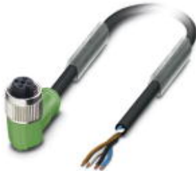
Sensor/Actuator cable, 4-position, PVC, Black RAL 9005, Free cable end, on Socket angled M12, A-coded, Cable length: 5 m
